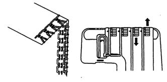
The looper loops are formed on the upper side: Tighten the lower looper tension (red), or loosen the upper looper tension (blue).
